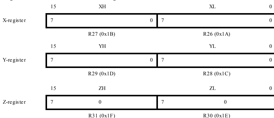
Figure 10-3 The X-, Y- and Z-Registers
